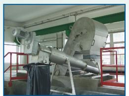
Extremly long service life due to special socket for fitting of screw
